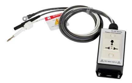
The TL-UP2 Test Adaptor allows for easy Hipot and Ground Bound connection to virtually any device with a power cord. The TL-UP2 routes high voltage to both the line and neutral pins of the power socket and connects the earth pin of the socket to the return of the tester. A separate test lead can be connected to the DUT chassis for continuity or Ground Bond testing to the earth pin of the DUT power cord. Available in Hipot/ Continuity or Hipot/ Ground Bond versions.
