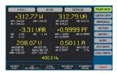
three different VPAs can exist in in a single PA900. In addition to the primary data, peak readings, phase, CF and other parameters are also available. Integrated data results (WHr) can also be controlled and viewed from the power data screen. For users with unique data requirements, custom data screens can be built with a spreadsheet application and downloaded to the PA900 via interface or USB drive.
