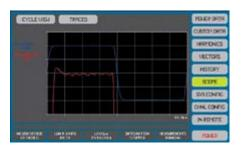
The cycle view represents a single cycle of the voltage and or current periodic waveforms. The above waveforms represent a full 10V square wave in blue and a 50:1 zoomed in view in red. Since the user sets amplitude and scaling - the result is an almost unlimited ability to amplitude zoom to expose fine detail. The sampling is forced to be asynchronous to higher order harmonics which leads to an effective sampling rate of 384MSPS.
