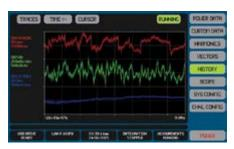
The PA900 automatically maintains a continuous historical record of all nonharmonic measurement results and selected harmonics. Up to four user selectable parameters can be graphically displayed using the HISTORY screen. The user can display the entire recorded period up to 397 days or zoom in as far as 1/64th of the total span. This provides an almost unlimited ability to amplitude zoom and includes a cursor which may be moved throughout the period with a touch of the screen.
