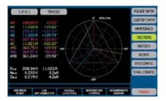
A polar chart graphically displays the fundamental voltage and current vectors for the selected channel or VPA. For multiphase VPAs, the inter-phase voltages and non-measured neutral phase vectors are displayed. The user may enable the display of and select the color of each vector up to a maximum of 10.
